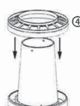
FIGURE 4 Pass the anti-waste ring through the cone and fix it to the tray.
